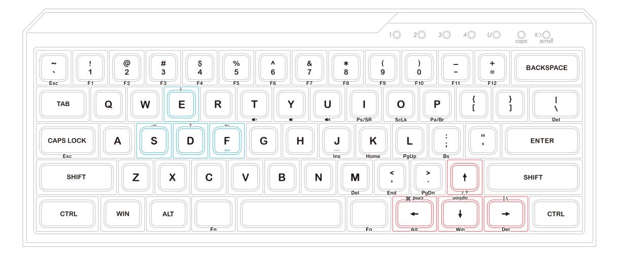
Remove top part of E/S/D/F with included special key puller and rotate bottom part 180 degrees and put top part of E/S/D/F back so that cursor symbols cannot be seen from typing position.
